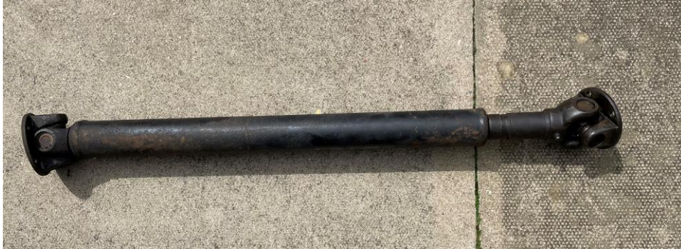
The yokes are incorrectly aligned.
