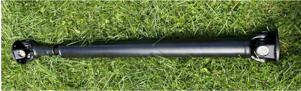
Completed propshaft with yokes correctly aligned.
